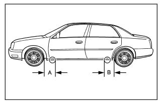
4. Find the jacking location from the diagram above and use the corresponding cutouts located in the plastic molding.
